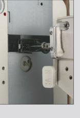
**Convenient bobbin thread check system** Thread remaining in the bobbin can be verified easily through inspection windows installed on the right side of board.
