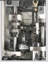
Simply structured thread trimming drive system
